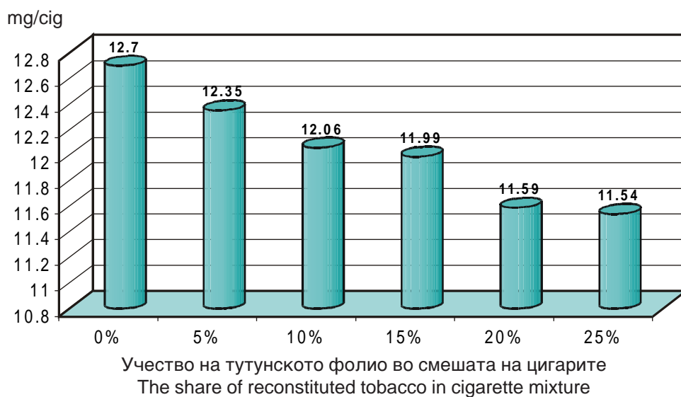
Fig. 12 The effect of reconstituted tobacco with cyclone dust on tar content in tobacco smoke
